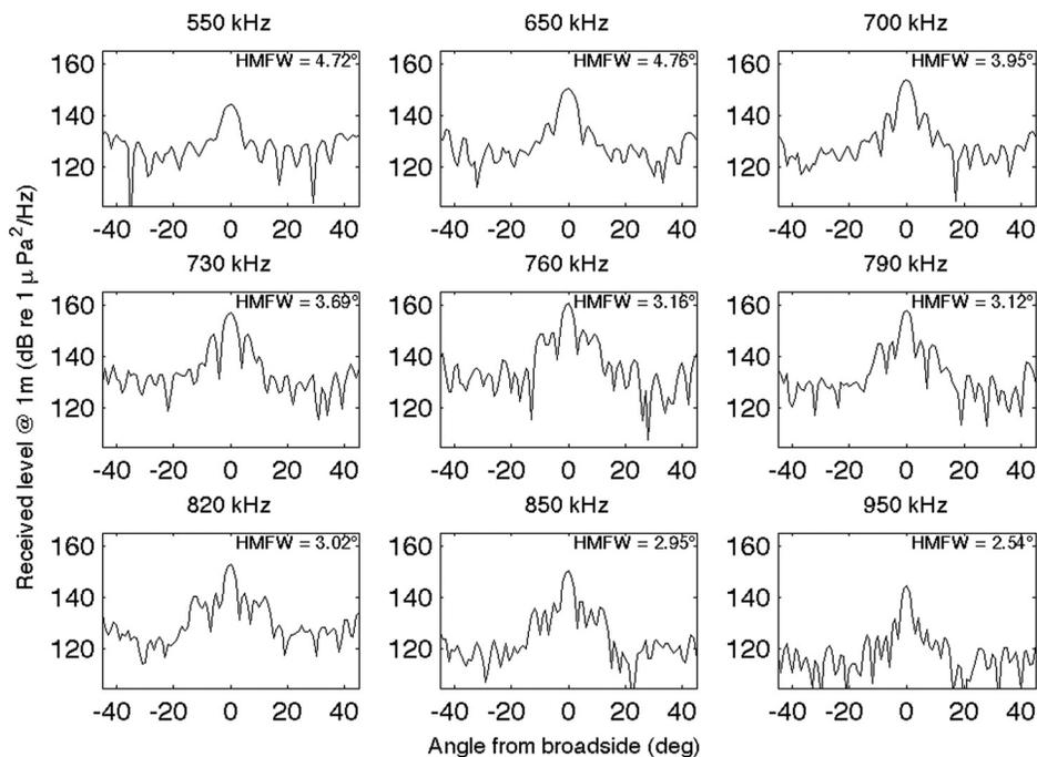
Fig. 2. Calibrated directivity plots of transmissions from the cylindrical transducer over a  $\pm 45^\circ$  deviation from broadside over the 550–950 kHz band. The half-maximum full width (HMFW) value of the main lobe in each case is shown on the upper right of each sub-plot.
