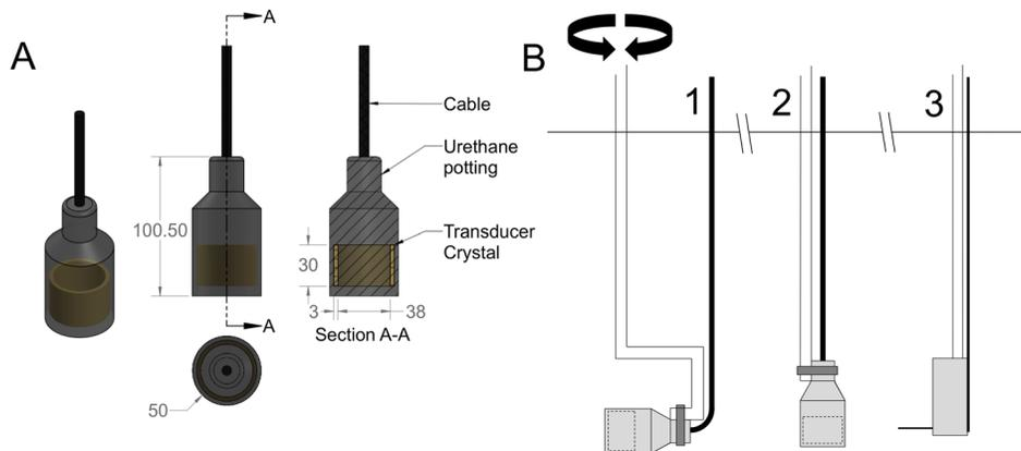
Fig. 1. (Color online) (A) A schematic of the hollow-cylinder transducer showing the dimensions and placement of the ceramic element in urethane potting material. (B) Schematic diagrams showing (B1) the transmission transducer, oriented horizontally, mounted to a rotating axis above the water line, (B2) a second (receive-only) cylindrical transducer mounted vertically, and (B3) the calibrated needle hydrophone.
