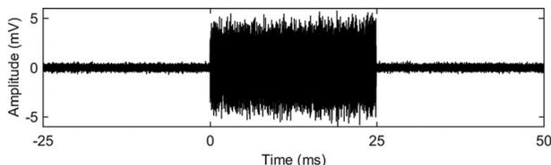
Fig. 4. High-pass filtered ( $f_c = 25$  kHz) time-series recording displaying a 25 ms communication packet and no discernible multipath from initial at-sea testing of the cylindrical transducer-cylindrical transducer system.
