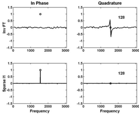
Figure 2. Numerical examples of the inversion of Eqn. 1. The top panels show the inversion of the 128 by 128  $\mathbf{W}$  matrix using equally spaced samples. The lower panels show the I1 inversion of the 128 by 2048  $\mathbf{W}$  matrix with randomly chosen time samples.
