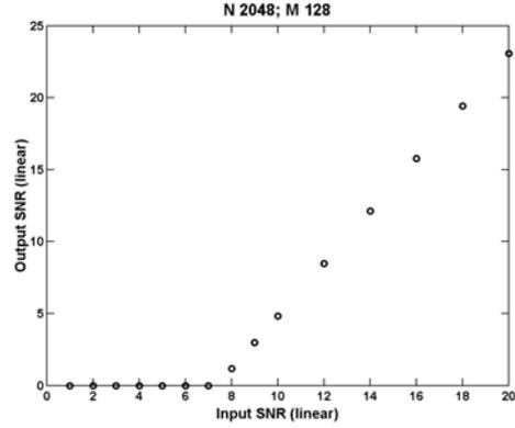
Figure 3. The output SNR as a function of input SNR with the number of frequency samples held constant at 2048 and the number of time samples at 128.
