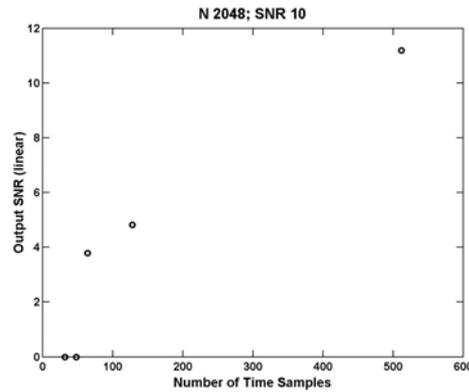
Figure 3. Comparison of output to input signal to noise ratios as a function of the number of random data samples.
