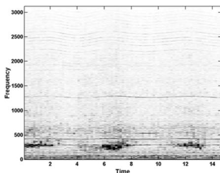
Figure 4. Spectrogram of a signal from one element of a towed array. The intensity is proportional to the absolute value of the spectrogram.
