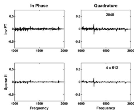
Figure 5. Comparison of the I2 inversion using 2048 data points with the coherent average of four I1 inversions using 512 data points. The vertical is linear.
