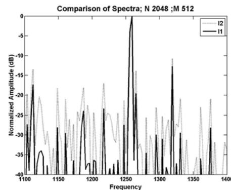
Figure 6. Comparison of the results shown in Fig. 5. The signals are compared with a dB scale. The peaks of each spectrum is normalized to one. The I2 spectrum is a dotted line and the I1 spectrum is a solid line.
