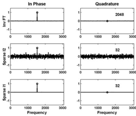
Figure 1. Numerical examples of inversion of Eqn. 1. The top panels show the inverse of full  $\mathbf{W}$ . The middle panels show the Moore-Penrose inverse and the bottom panels show the l1 inversion. The in-phase and quadrature components are displayed to show the phase.
